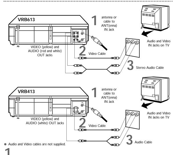
Connect the antenna or cable to the ANT(enna) IN Jack on the back of the VCR.
